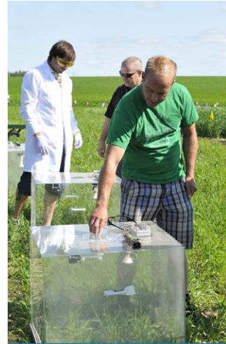
A demonstration of the gas chambers for N 2 O emissions sample collection on Richard Farrell's plot
