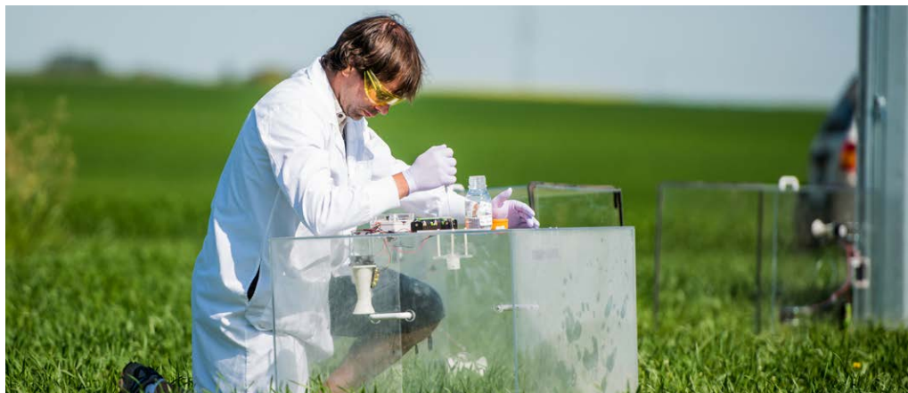
Darin Richman demonstrating a sample measurement for N_2O emissions from the gas chamber
