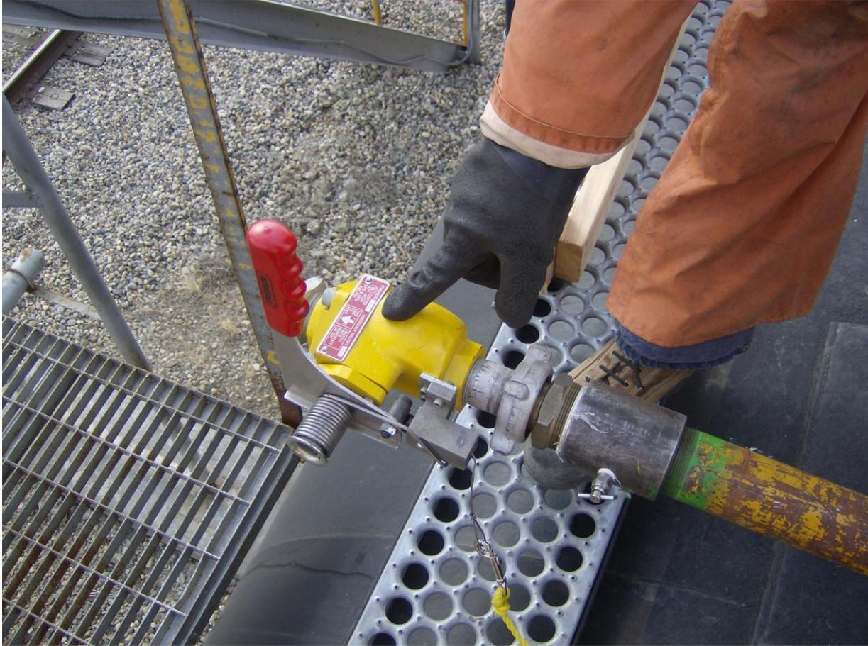
**Emergency shut-off valve on a rail car.**
