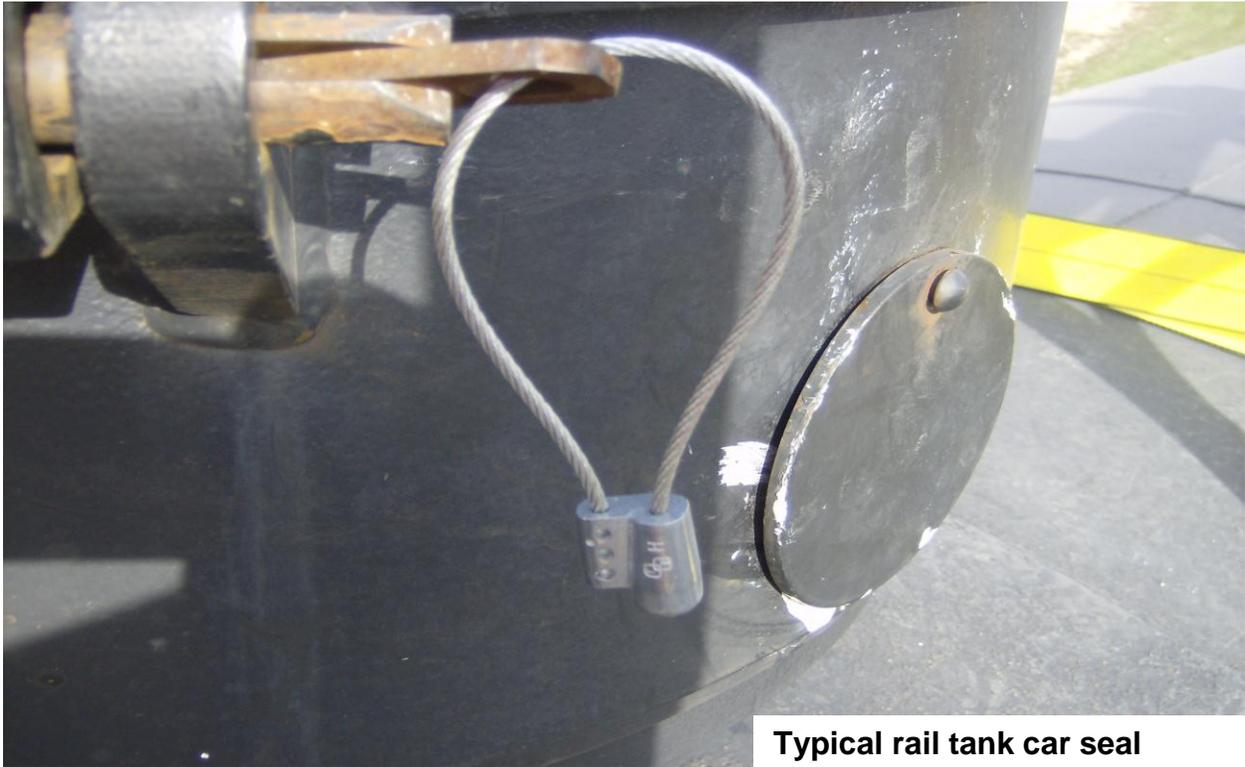
**Typical rail tank car seal**
