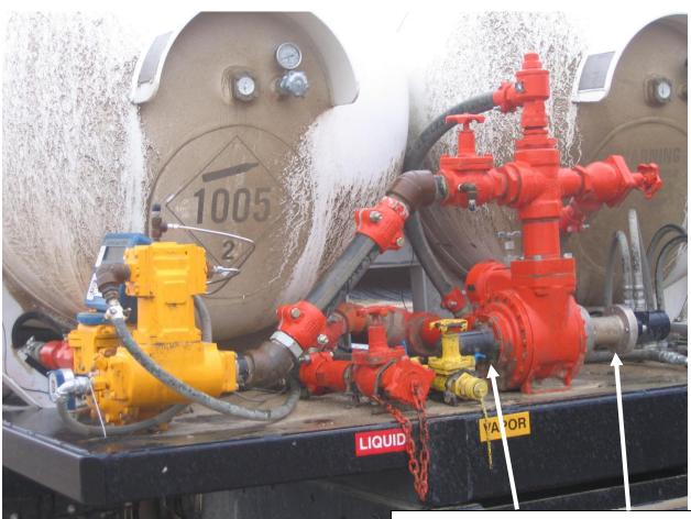
Approved anhydrous ammonia pump, securely mounted with guards both sides of pump.
