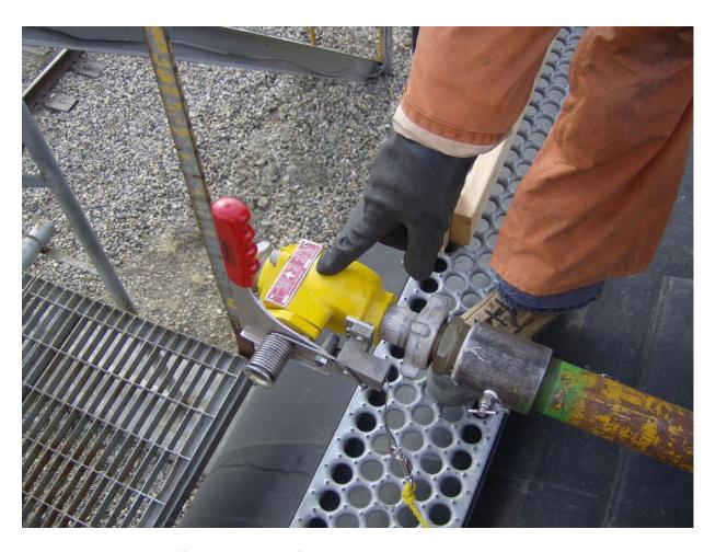
Emergency shut-off valve on a rail car.
