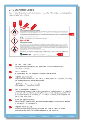
Fig 2. New GHS Sample SupplierLabel
