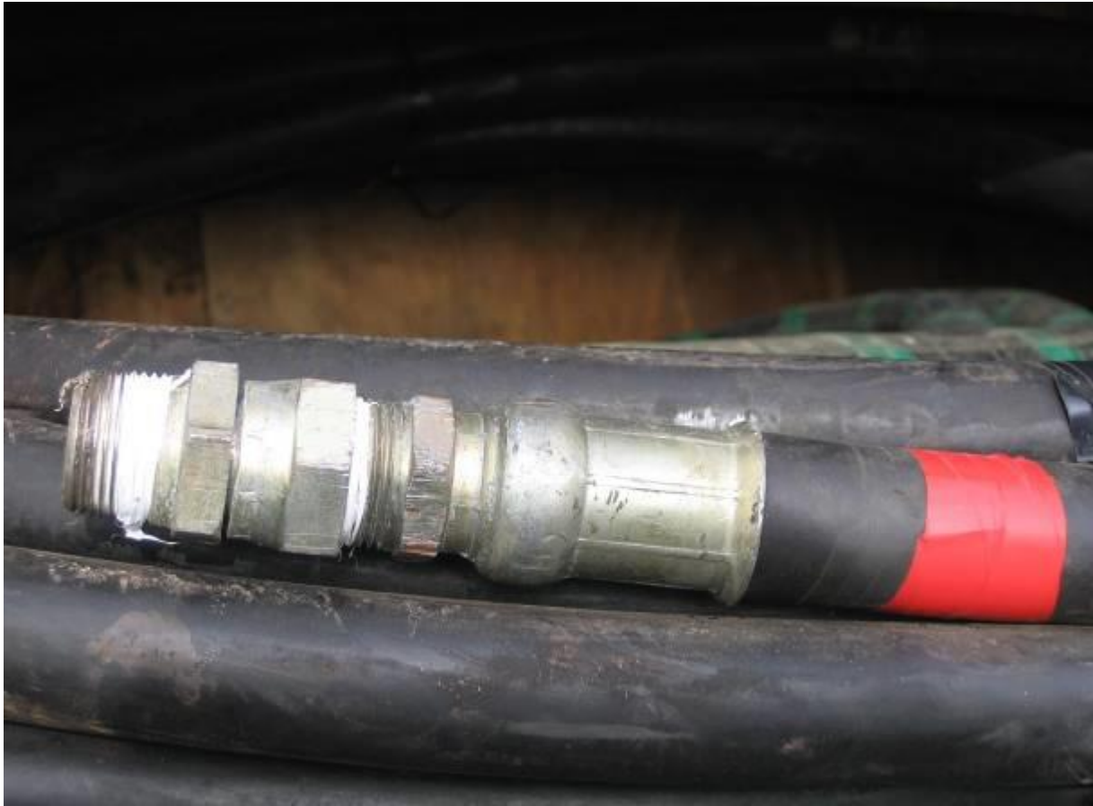
Figure 10. Crimp on hose Fittings
