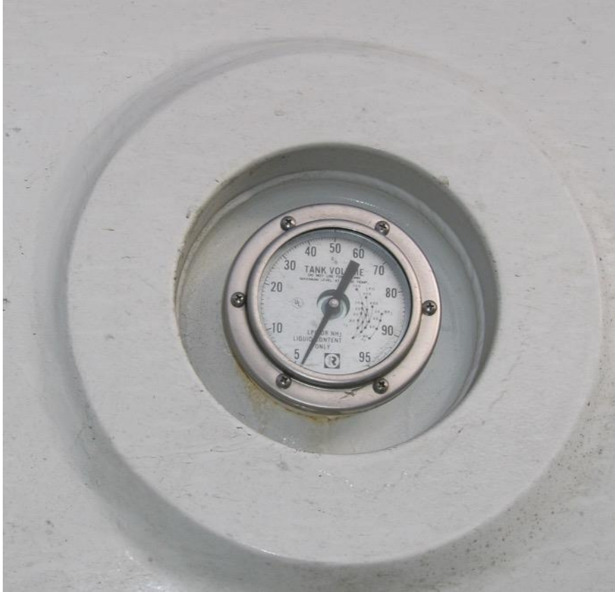
Fixed liquid level gauge. Disadvantage: Only indicates 85% level. Releases product.
