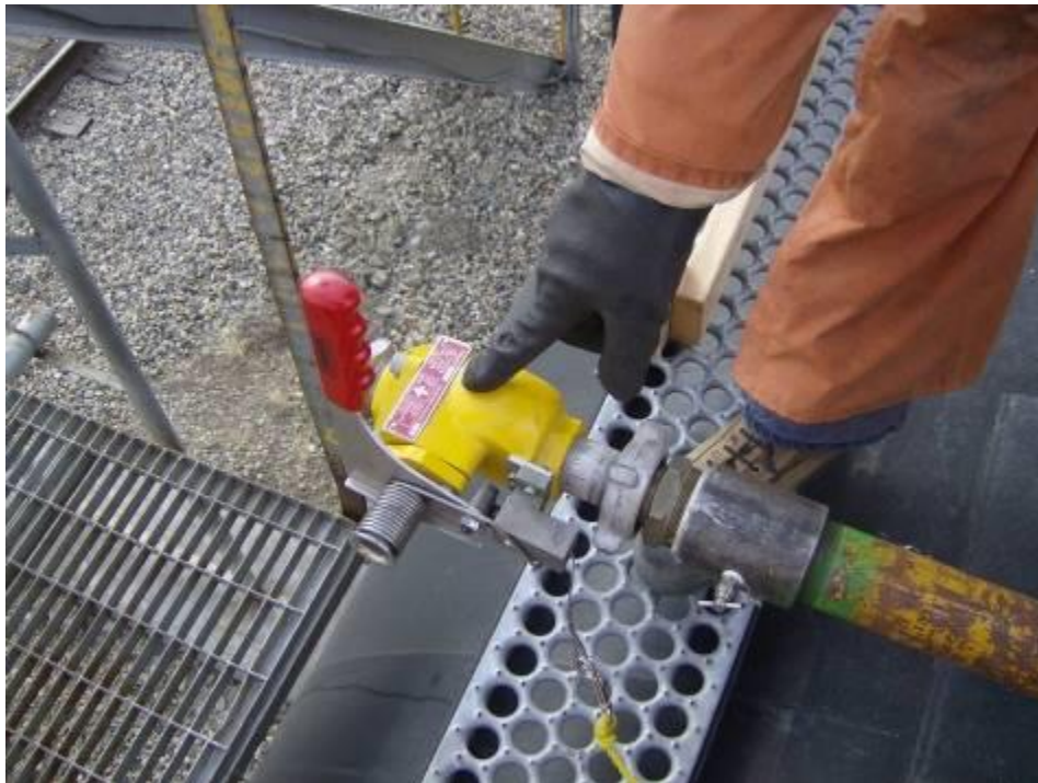
Figure 2. Emergency shut-off valve on a rail car.
