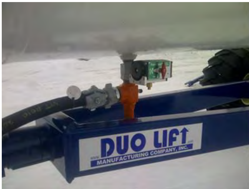
Figure 3: Example of a shut down system installed on a tank
