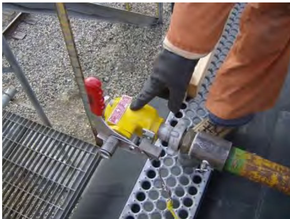
Figure 2. Emergency shut-off valve on a rail car.
