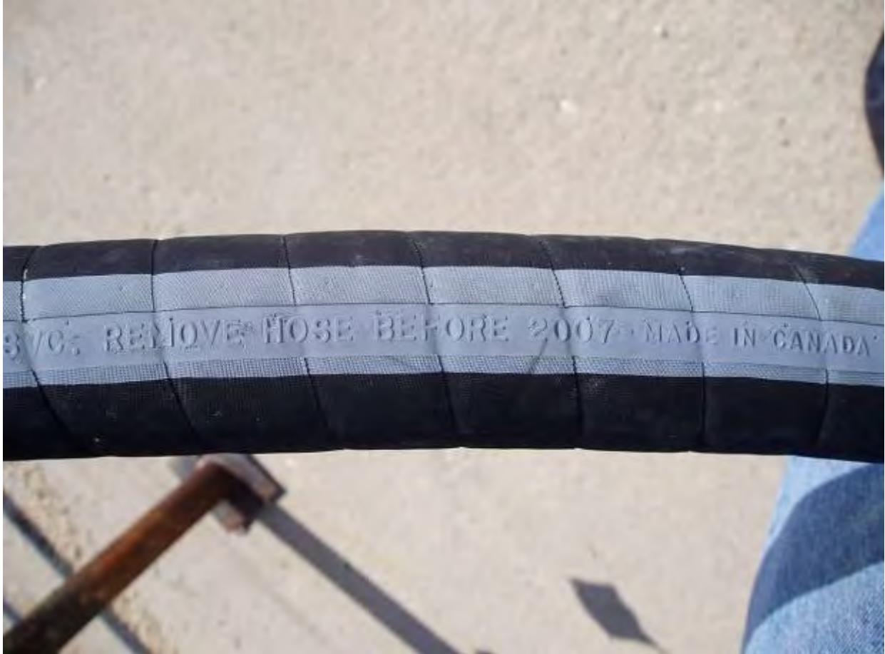
Figure 8. Hoses Marked for Remove from Service Date
