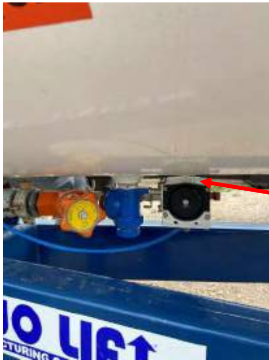
Figure 2: Example of an air actuated shut down system
