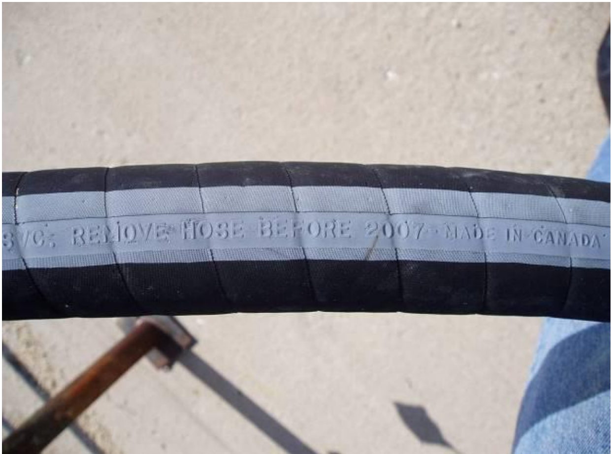
Figure 8. Hoses Marked for Remove from Service Date
