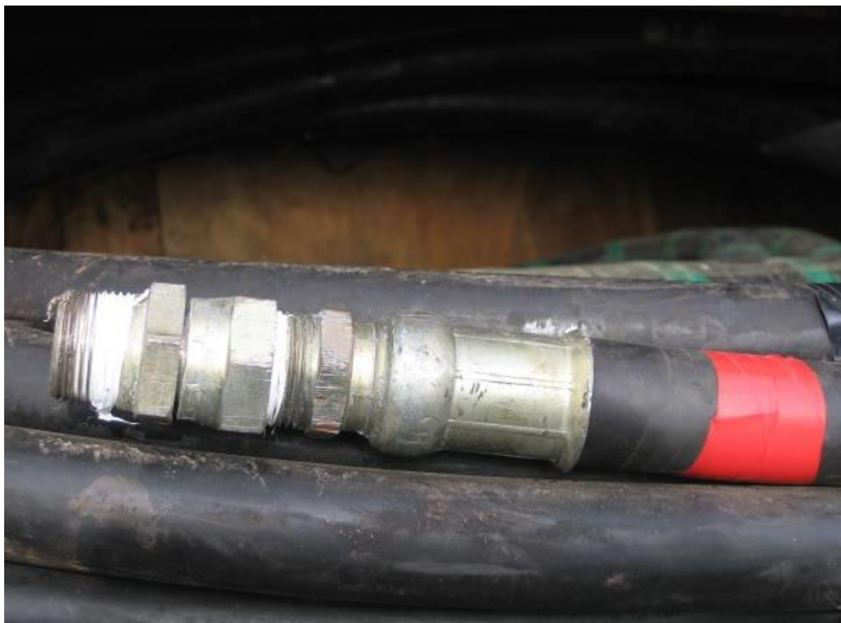
Figure 10. Crimp on hose Fittings
