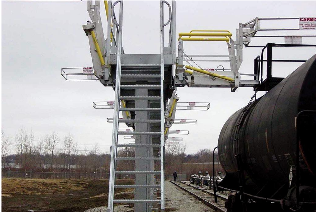
Figure 5. Example Fall Restraint System
