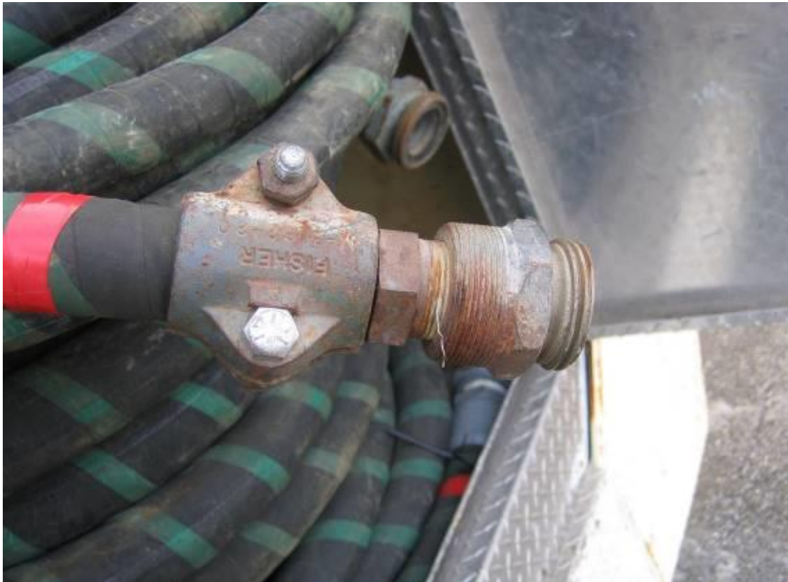
Figure 9. Bolt on hose Fittings
