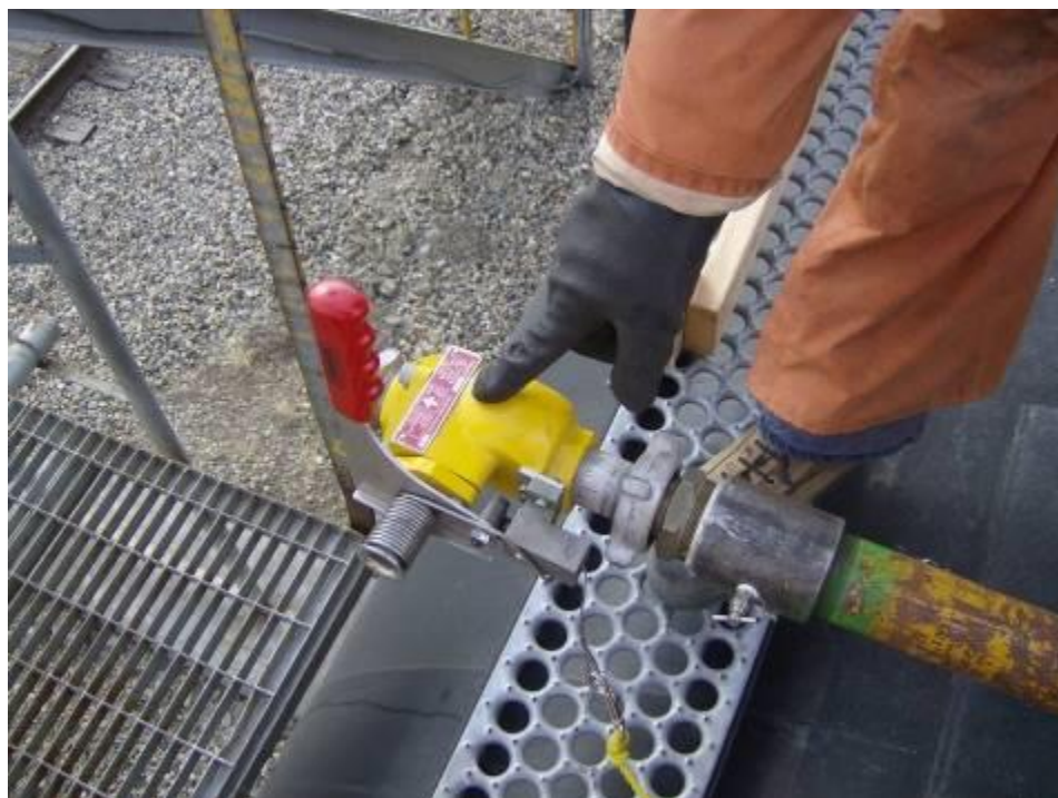
Figure 2. Emergency shut-off valve on a rail car.
