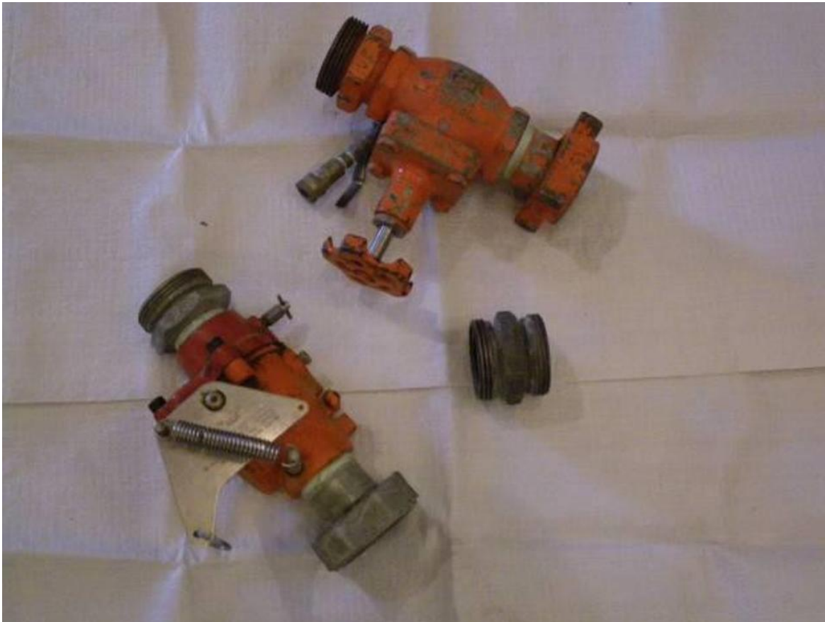
Figure 3. Valves suitable for anhydrous ammonia service through a visual inspection of the equipment.
