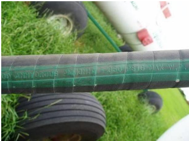
Figure 7. HOSES – Marked Approved for Anhydrous Ammonia and MAWP
