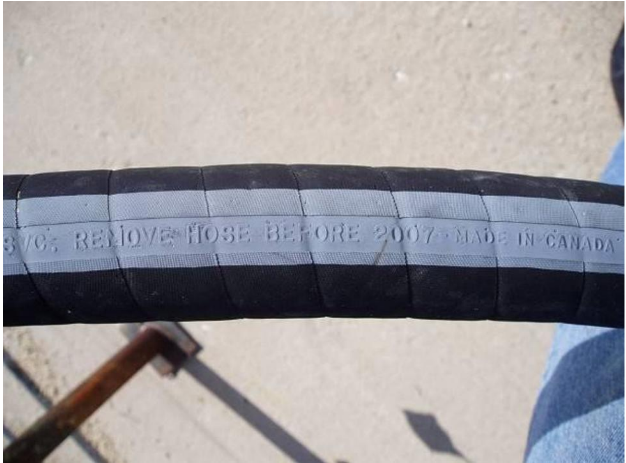
Figure 8. Hoses Marked for Remove from Service Date
